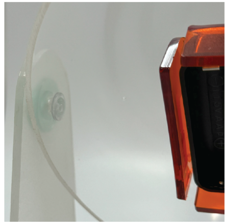
The acrylic is prone to cracking so it required more support when drilling holes than the PET. Because of this, there was some minor cracking that occurred when we were drilling the side holes.
