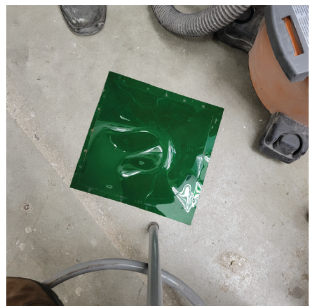
The coloured acrylic did not vacuum form, therefore the intended colours of the design had to change.
