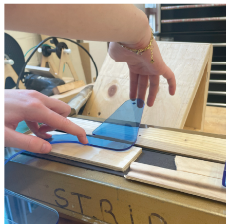
The coloured plastic took longer to melt on the strip heater than the clear plastic.
