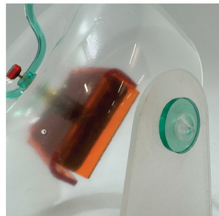
The fasteners were too long so we had to laser cut spacers to hold it in place.
