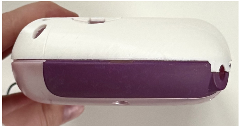
Figure 15: Side view of final 3D print, good fit and seamless curvature. Source: Author
