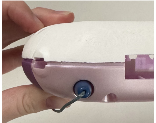
Figure 13: Top view of final 3D print, gap created by inner rib fit. Source: Author
