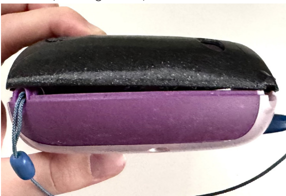
Figure 10: Side view of initial 3D print, hole cut out is missing. Source: Author
