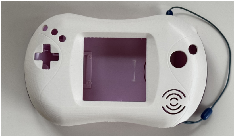
Figure 12: Front view of final 3D print, fits well on bottom housing. Source: Author
