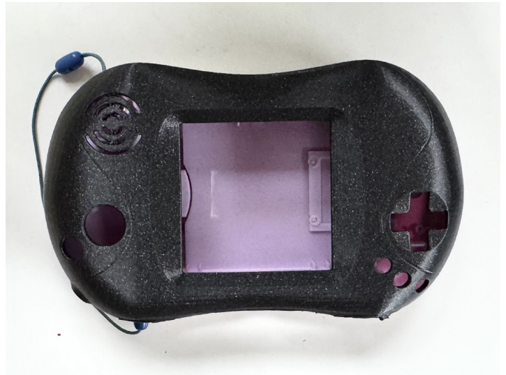
Figure 8: Top view of initial 3D print. Source: Author
