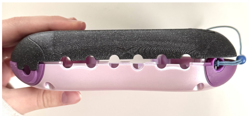
Figure 11: Bottom view of initial 3D print, button holes are not matching up in some instances. Source: Author
